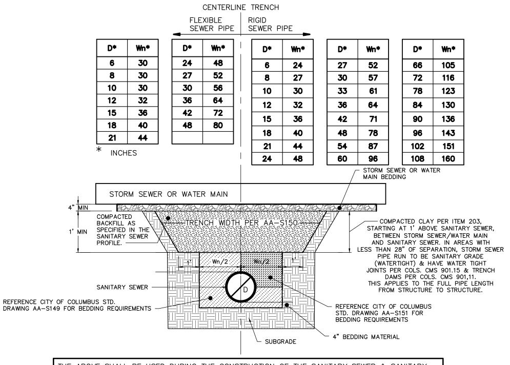
THE ABOVE SHALL BE USED DURING THE CONSTRUCTION OF THE SANITARY SEWER & SANITARY SERVICE LATERALS AT EXISTING/PROPOSED STORM SEWER & ALL WATERLINE CROSSINGS. IF IT IS DISTURBED DURING CONSTRUCTION OF THE STORM SEWER OR THE WATERLINE, IT MUST BE RESTORED TO THE REQUIREMENTS OF THE DETAIL. LENGTH OF THE I/I BARRIER PROTECTION FOR SANITARY MAINS AND/OR LATERALS SHALL BE 10 FEET CENTERED ON STORM/WATERLINE PIPE CROSSING AND MEASURED ALONG THE SANITARY MAINLINE OR SERVICE LATERAL.
